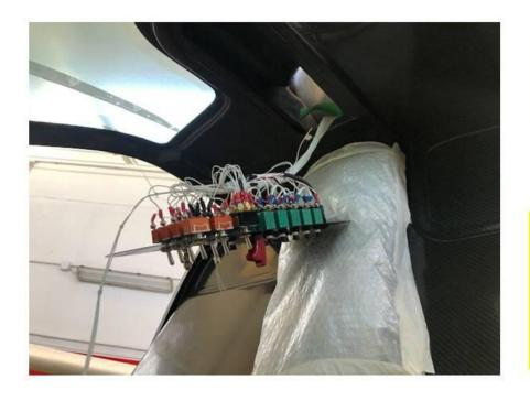
Step 1-remove the switch panel
