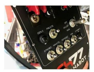
\* Step 5- Cut both cables connected to GEN 2 switch ,Remove GEN2 switch and reconnect them both cable to the button switch, no problem if you reverse the phase
