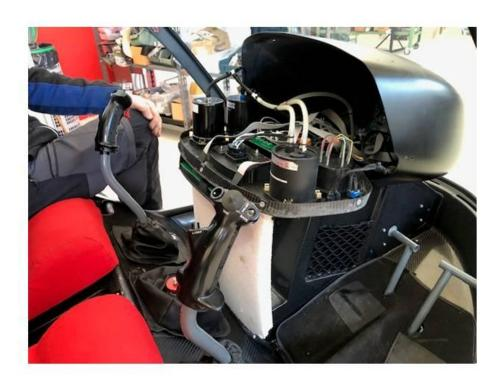
Step 7Unscrew the instrument panel, and place a suitable support for the panel
